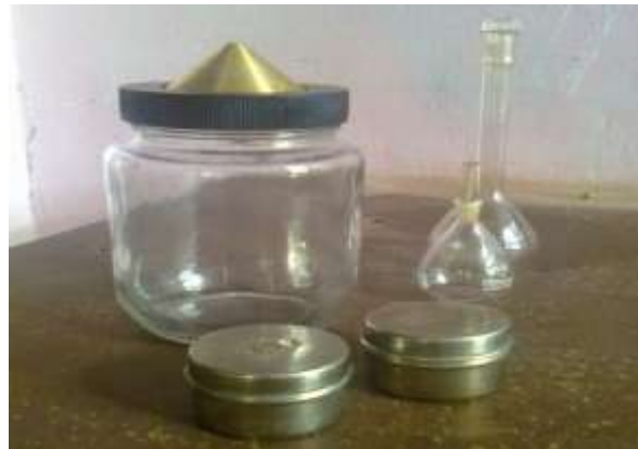
Fig. 2 Specific Gravity Apparatus
