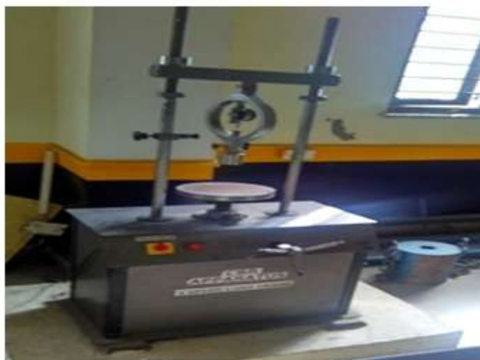
Fig. 4 California Bearing Ratio Test
